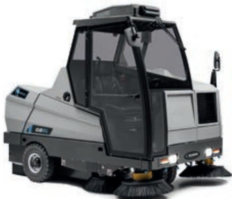
OBBL Direct load, front guide with Bullsistem® technology Cleaning path 1270/2100 mm
